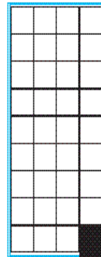
Example of full-cell shading that can reduce PV module power by \frac{1}{2}
